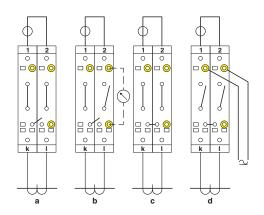
Simple current transformer test circuit
