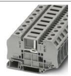
Test disconnect terminal block, With test socket screws for insertion of test plugs, Connection type: Bolt connection, Cross section: 0.1 mm² - 6 mm², AWG: 26 - 10, Nominal current: 41 A, Nominal voltage: 500 V, Length: 82.4 mm, Width: 12.3 mm, Color: gray, Assembly: NS 35/7,5, NS 35/15
