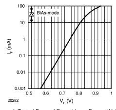
Figure 4. Typical Forward Current  $\rm I_F$  vs. Forward Voltage  $\rm V_F$
