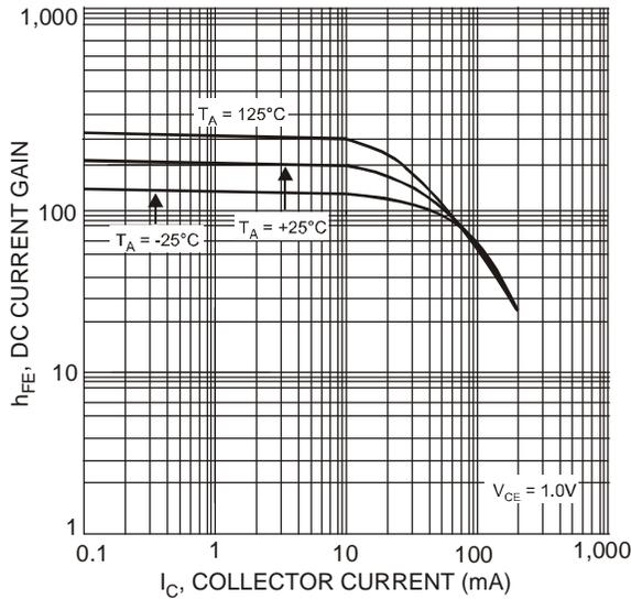
Fig. 1 Typical DC Current Gain vs. Collector Current
