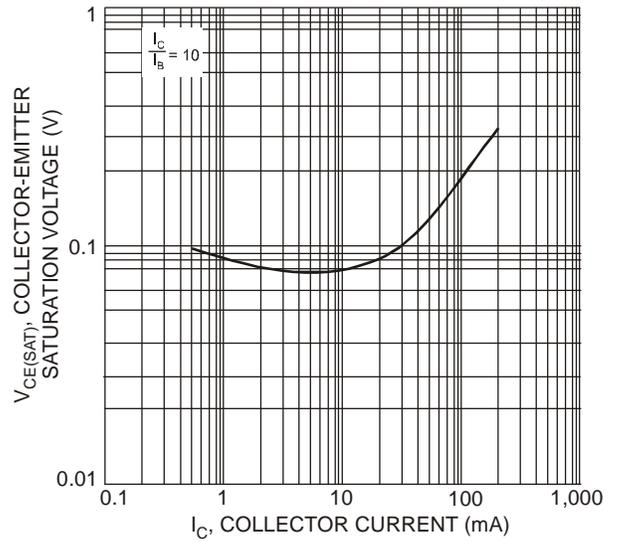
Fig. 2 Typical Collector-Emitter Saturation Voltage vs. Collector Current
