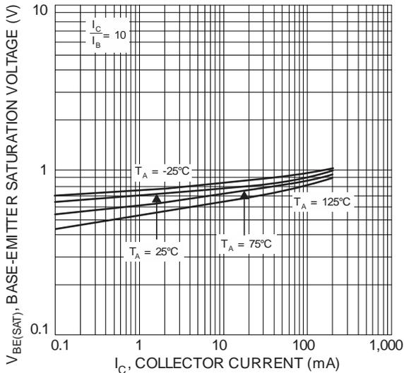
Fig. 3 Typical Base-Emitter Saturation Voltage vs. Collector Current
