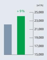
Comparison figures measured in application, each with 800 mm EC fan. AxiTop is currently available for ebm-papst axial fan sizes 800mm and 910mm.
