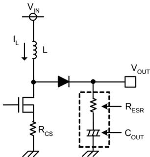
Output capacitor needs to be selected in consideration of equivalent series resistance required to even the stable area of output voltage or ripple voltage. Be aware that set LED current may not be flown due to decrease in LED terminal voltage if output ripple component is high.
