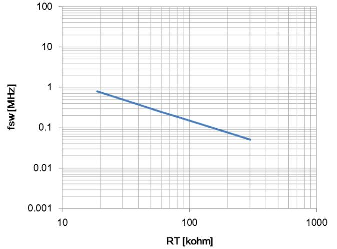
Figure 8. Fsw vs RT characteristic
