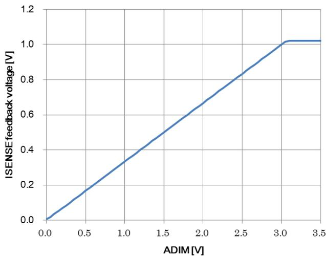
Figure 11. ISENSE feedback voltage vs ADIM voltage characteristic
