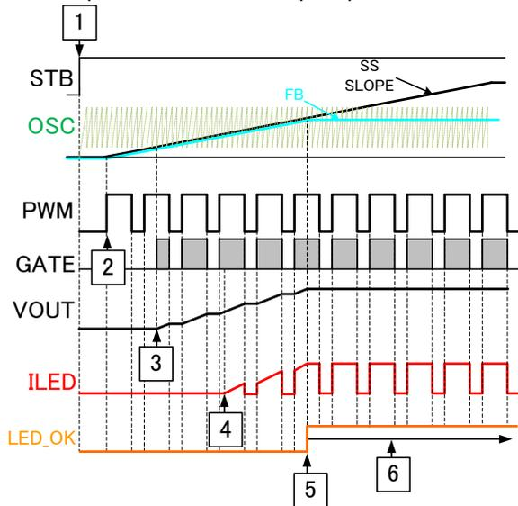
Figure 20. Startup waveform
