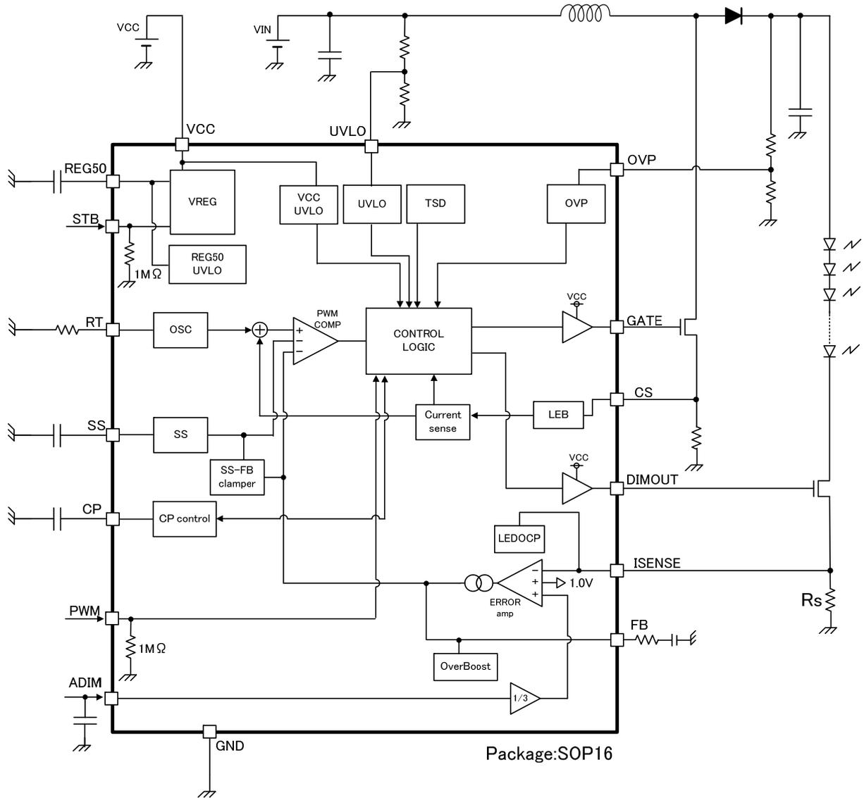
Figure 6. Block Diagram
