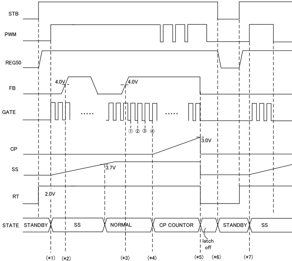
Figure 37. FBMAX Detection
