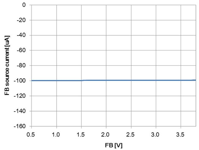
Figure 10. FB source current vs FB voltage characteristic
