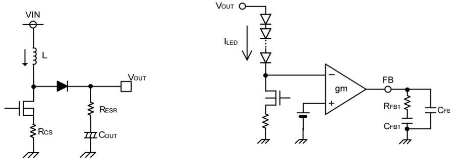
Figure 31. Output stage and error amplifier diagram
