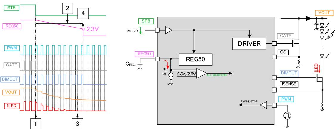
Figure 22. The waveform and diagram at shutdown
