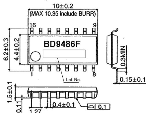
Figure4. Physical Dimension and Marking Diagram of SOP16
