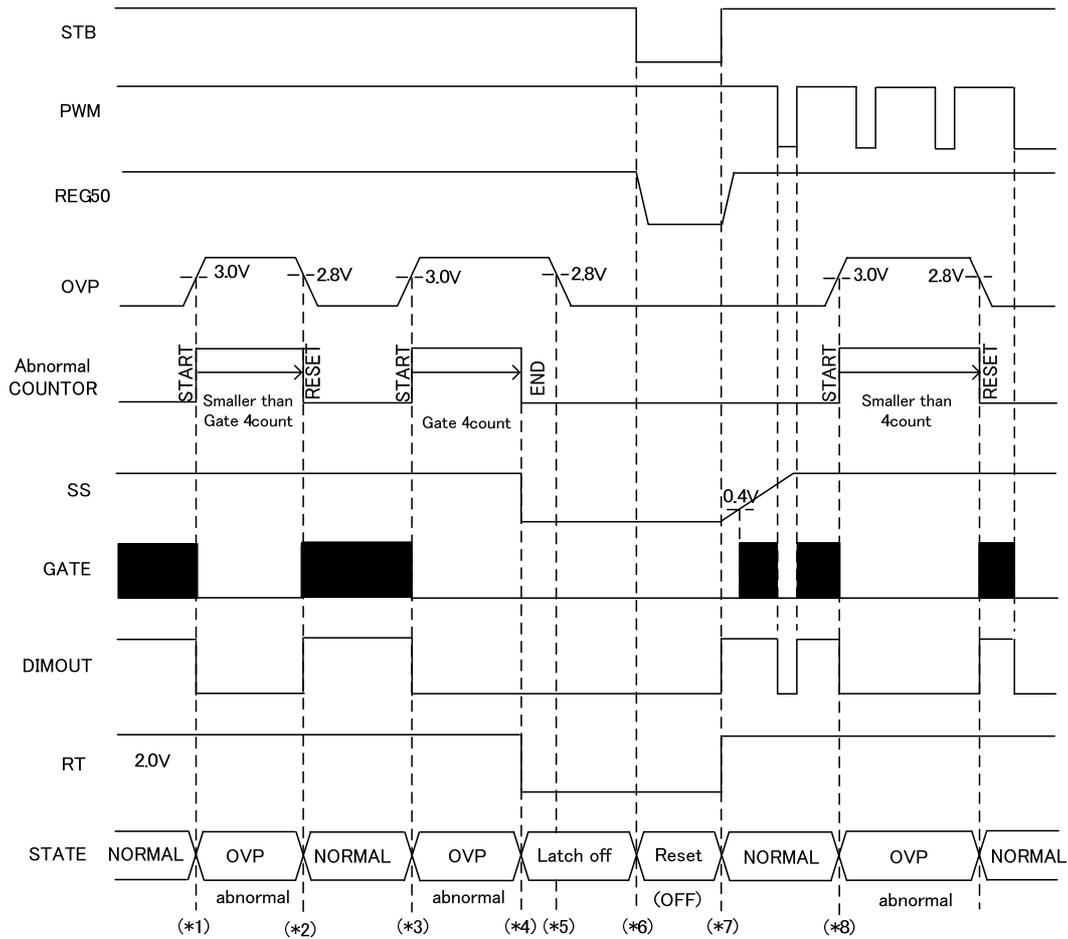
Figure 36. OVP Detection
