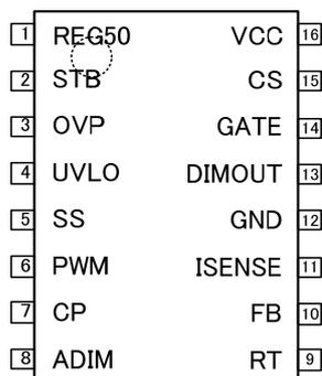
Figure 3. Pin Configuration
