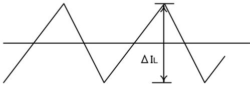
$$\Delta I_L = \frac{(V_{OUT}[V] - V_{IN}[V]) \times V_{IN}[V]}{L[H] \times V_{OUT}[V] \times f_{SW}[Hz]} \quad [A]$$
