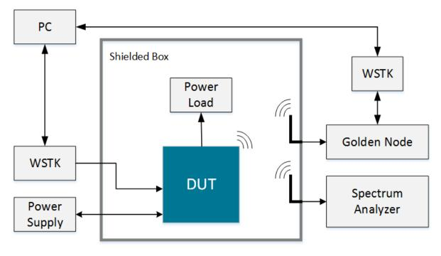
Figure 10.1. Test System Diagram
