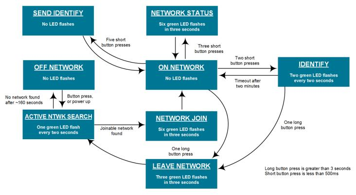
Figure 5.1. Device Operation State Diagram
