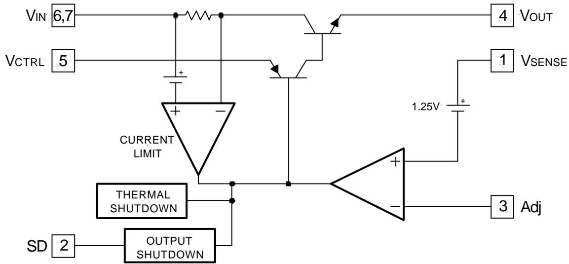
Figure 2 - Simplified block diagram of the IRU1176.
