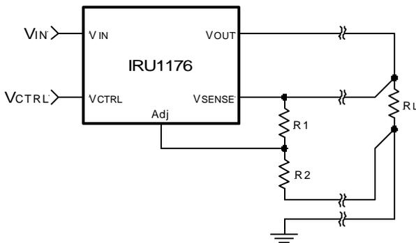
Figure 4 - Schematic showing connection for best load regulation.
