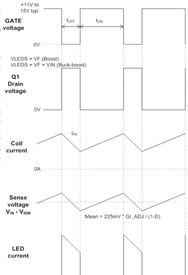
**Figure 24 Operating Waveforms (Boost and Buck-Boost modes)**
