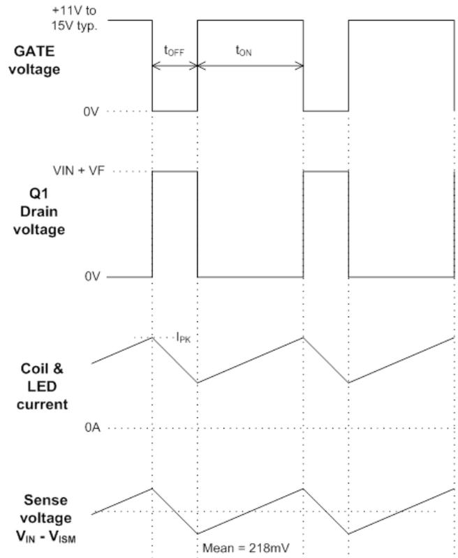
Figure 22 Operating Waveforms (Buck Mode)
