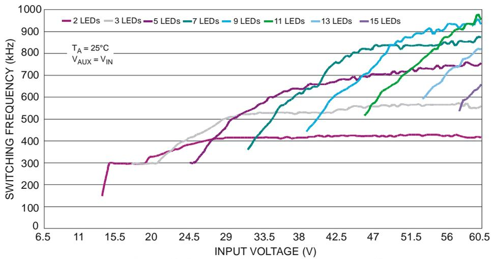
Figure 13 Frequency ZXLD1370 - Buck Mode -  $L=47\mu H$
