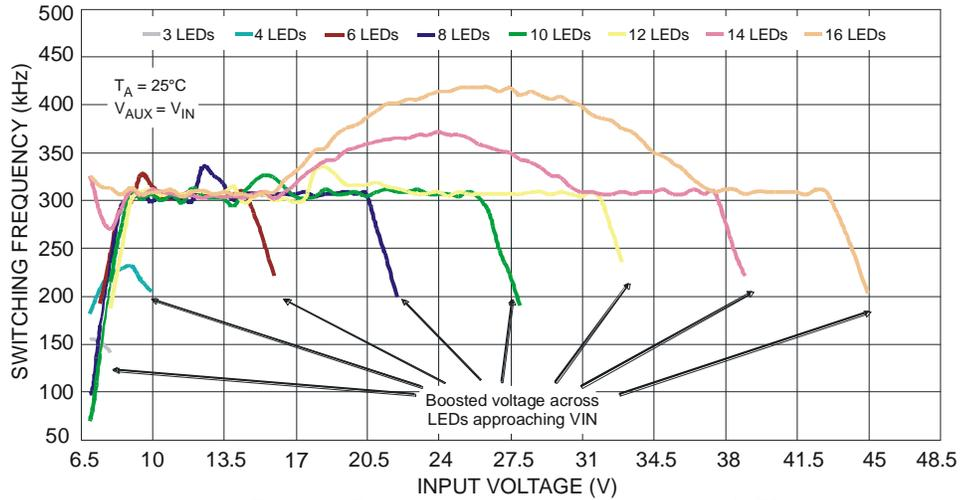
Figure 16 Frequency vs. Input Voltage & Number of LED
