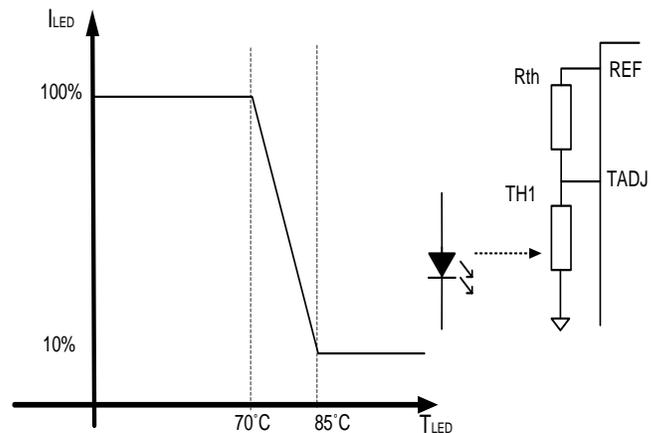
Thermal network response in Buck configuration with:
