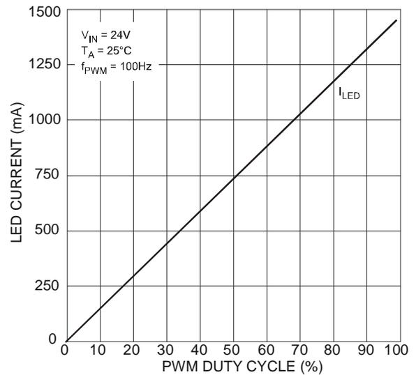
Figure 4 I<sub>LED</sub> vs. PWM Duty Cycle
