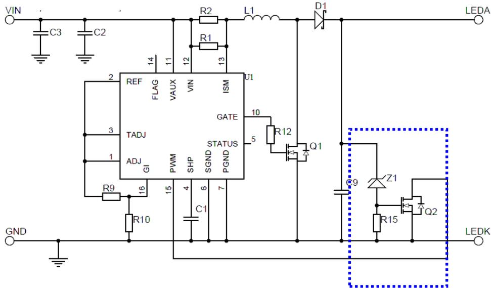
**Figure 38 OVP Circuit**
