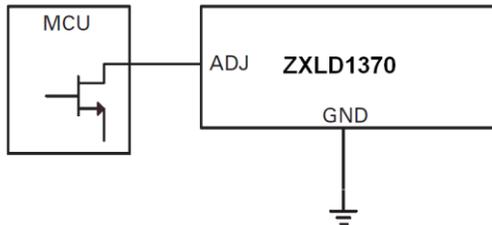
**Figure 31 PWM Dimming from MCU**
