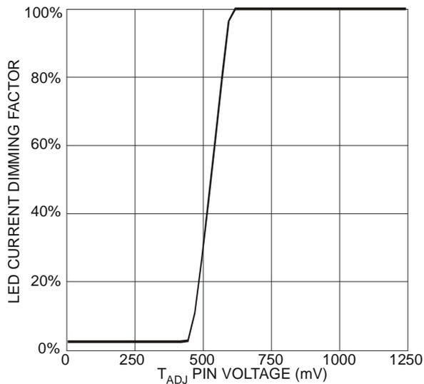
Figure 3 LED Current vs. T<sub>ADJ</sub> Voltage
