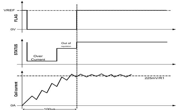
**Figure 36 Diagnostic During Start-Up**
