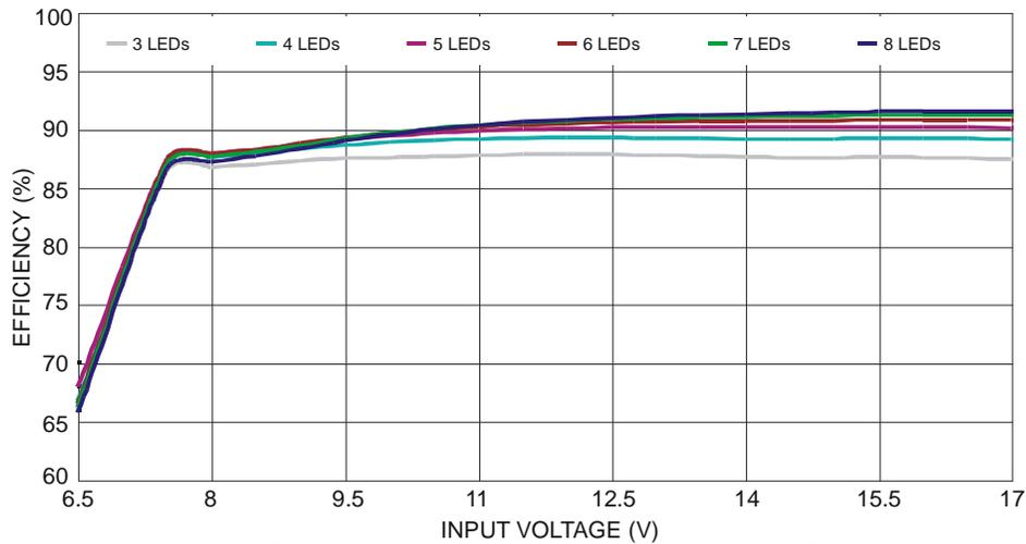
Figure 20 Efficiency vs. Input Voltage & Number of LED
