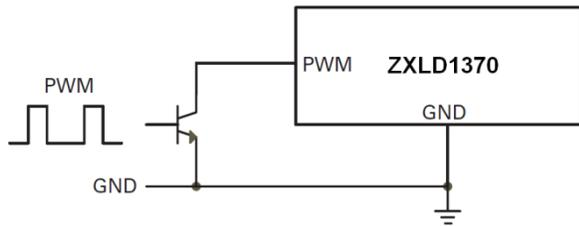
**Figure 30 PWM Dimming from Open Collector Switch**
