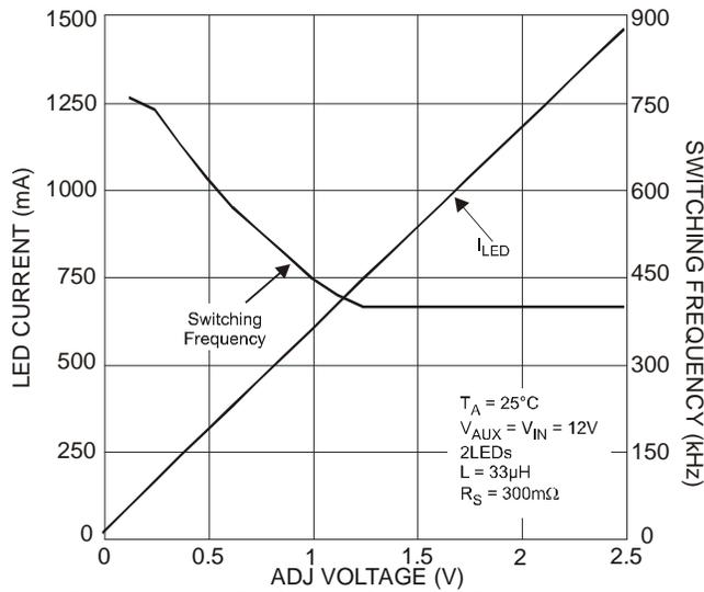
Figure 5 Buck LED Current, Switching Frequency vs.  $V_{ADJ}$
