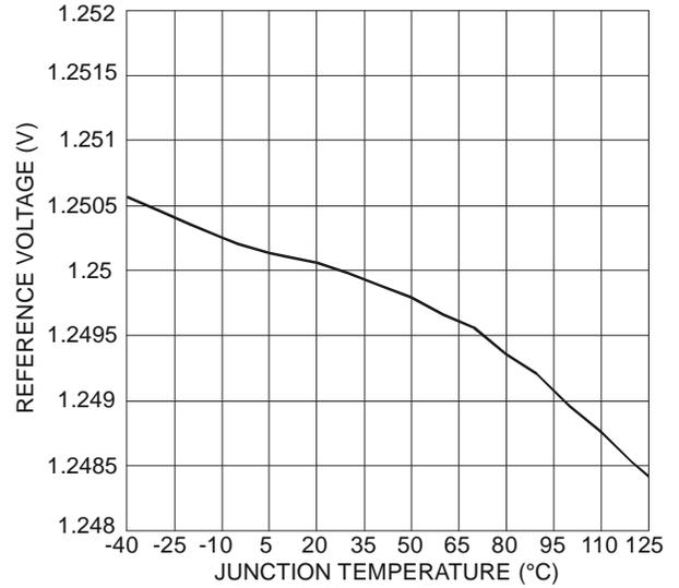
Figure 2 V<sub>REF</sub> vs. Temperature
