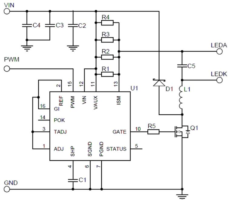
**Figure 40 Application Circuit: 2.8A Buck LED Driver**
