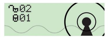
In scanning mode the display will display the total number of both non-encrypted and encrypted Wi-Fi signals detected.
