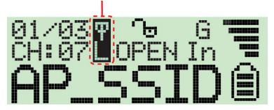
In "lock mode" the detector constantly refreshes the signal strength so the user can move around to find where the detected signal strength is the strongest.
