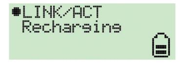
The battery strength indicator will be animated while the Wi-Fi detector is being recharged.
