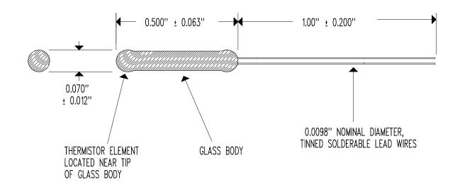
RESISTANCE @  $+25^{\circ}$ C = 1,000  $\Omega$  ± 5% RESISTANCE/TEMPERATURE CURVE = "E" BETA " $\beta$ " (+25 TO +85°C) = 3,348°K NOMINAL TEMPERATURE COEFFICIENT @  $+25^{\circ}$ C = -3.67%/°C NOMINAL TEMPERATURE RATING = -50 TO  $+300^{\circ}$ C
