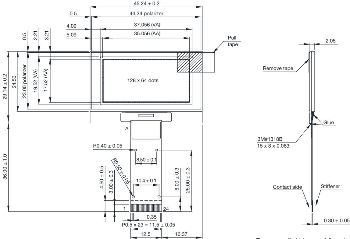
The non-specified tolerance of dimension is  $\pm 0.2$  mm
