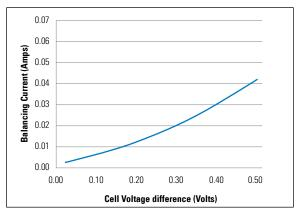
Figure 2. Balancing current versus cell volage differential.
