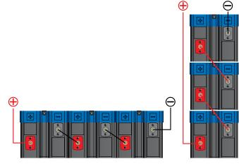
Figure 6. Series connected modules (horizontal or vertical). In this example, the system would provide 30KW for 15 seconds at 168V.
