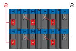
**Figure 8.** 3 Series x 2 Parallel connect modules. In this example, the system would provide 60KW for 15 seconds at 168V. Parallel cables (dashed lines) connecting modules in the middle are optional.
