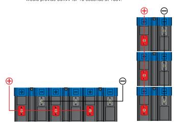
Figure 7. Parallel connected modules (horizontal or vertical). In this example, the system would provide 30KW for 15 seconds at 56V.
