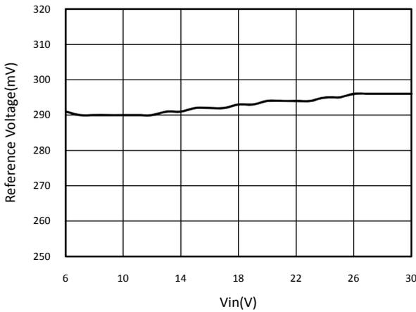
**Figure 10** V<sub>FB</sub> voltage vs. Vin
