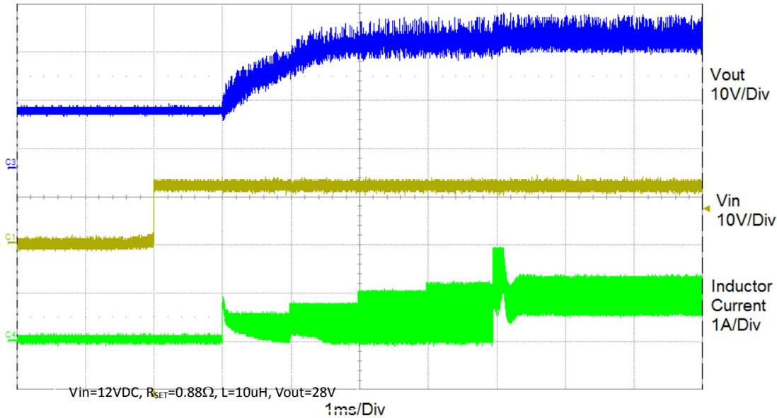
**Figure 11** Soft-start waveform
