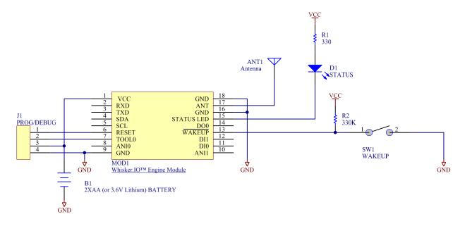
The Whisker.IO Engine is essentially a wireless IoT sensor in a module. Because it can measure temperature internally, all that is required to turn the module into a complete wireless temperature sensor is battery power and an antenna.
