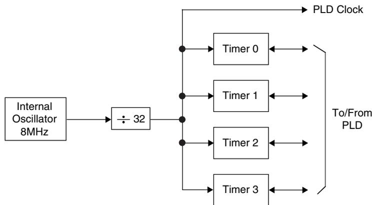
The internal oscillator runs at a fixed frequency of 8 MHz. This signal is used as a source for the PLD and timer clocks. It is also used for clocking the comparator outputs and clocking the digital filters in the voltage monitor circuits.
