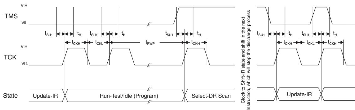
Figure 8. Verify Timing Diagram
