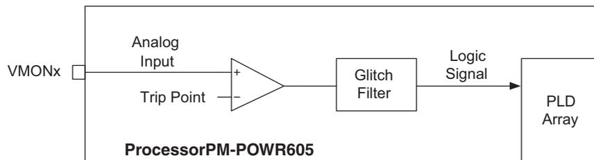
Figure 10 shows the functional block diagram of one of the six voltage monitor inputs - 'x' (where  $x = 1 \dots 6$ ). Each voltage monitor can be divided into two sections: Analog Input, and Filtering.
