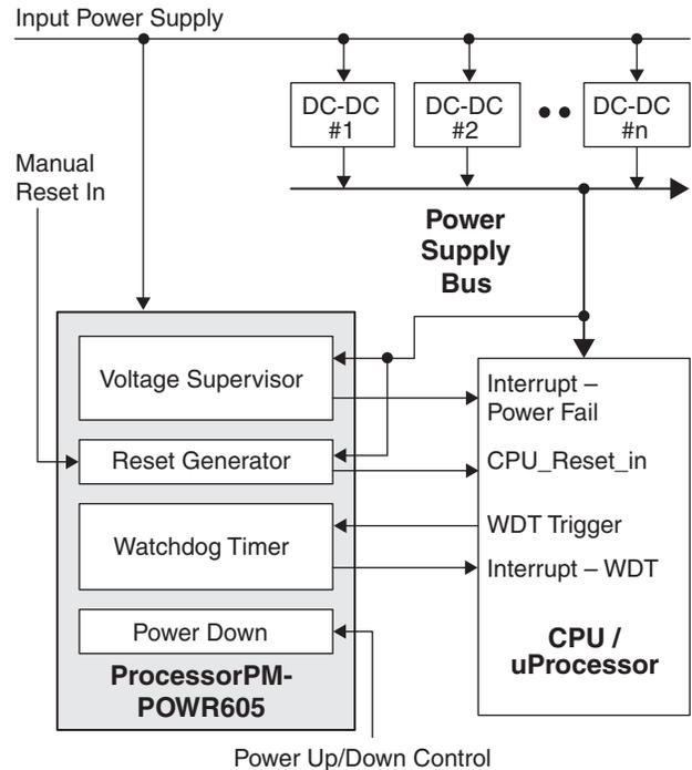
The diagram above shows how a ProcessorPM-POWR605 is used in a typical application. It controls power to the microprocessor system, generates the CPU reset and monitors critical power supply voltages, generating interrupts whenever faults are detected. It also provides a watchdog timer function to detect CPU operating and bus timeout errors.
