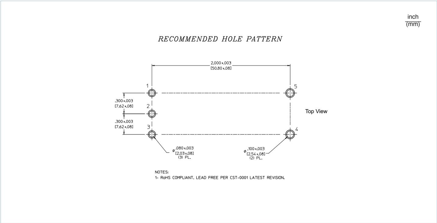
Figure 35 — IBC PCB recommended hole pattern
