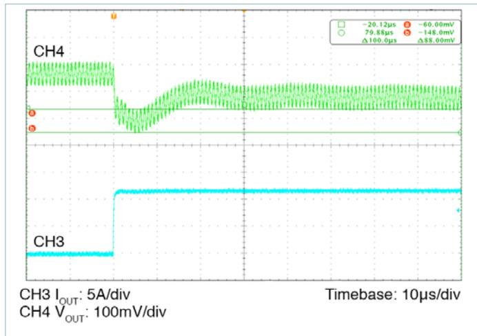
Figure 12 — Load transient response; nominal line, load step 75-100%
