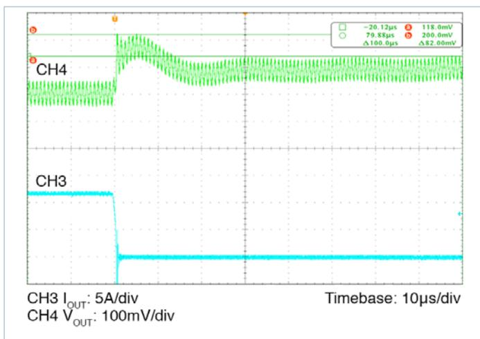
Figure 15 — Load transient response; nominal line
