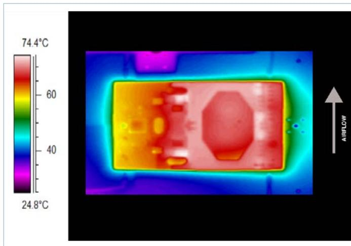
Figure 30 — Thermal plot, 600LFM, 25°C, 48V<sub>IN</sub>, 600W output power
