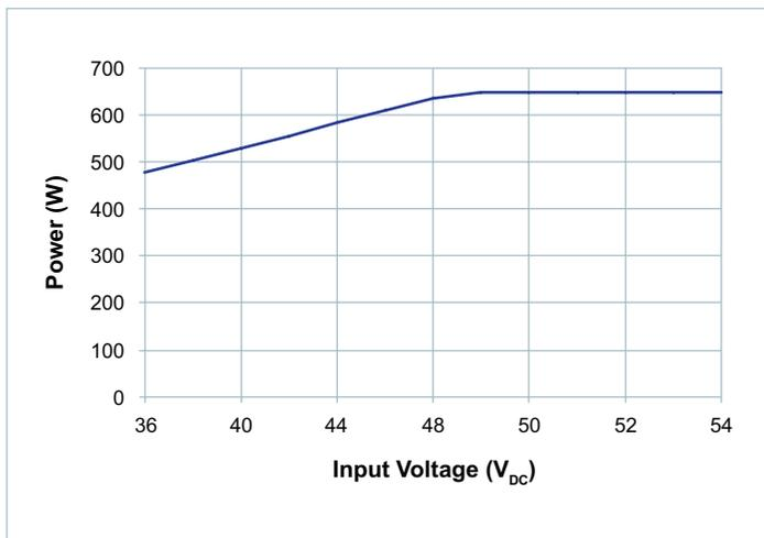
Figure 22 — Maximum output power vs. input voltage
