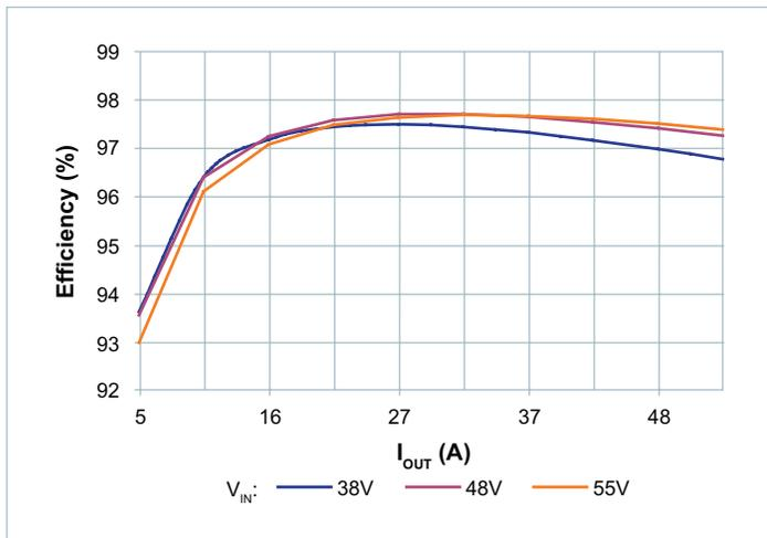
Figure 1 — Efficiency vs. output current, 25°C ambient
