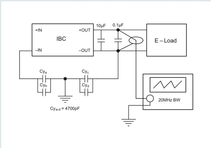
Figure 25 — Test circuit; output voltage ripple
