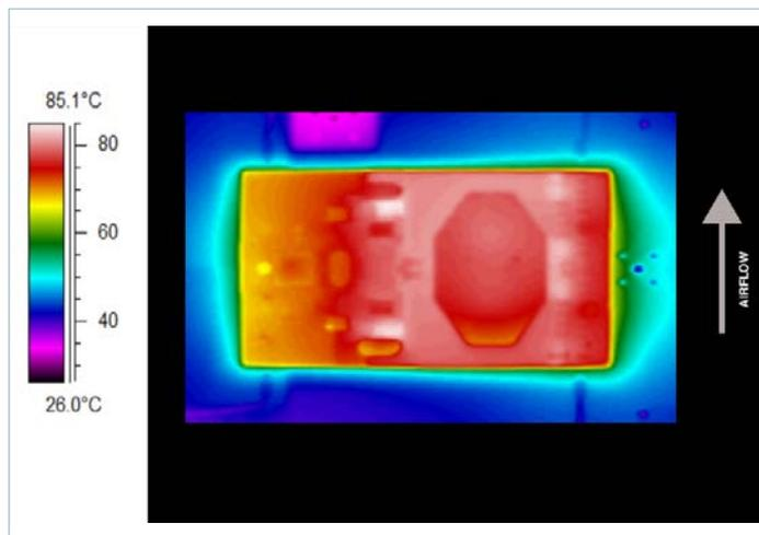
Figure 28 — Thermal plot, 400LFM, 25°C, 48V<sub>IN</sub>, 600W output power
