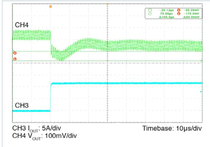
Figure 14 — Load transient response, nominal line
