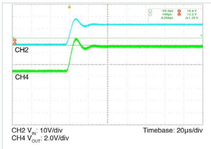
Figure 16 — Input transient response;
