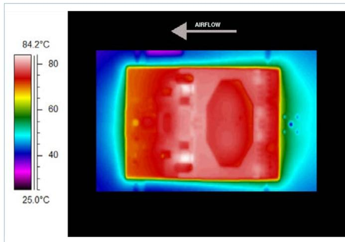
Figure 31 — Thermal plot, 600LFM, 25°C, 48V<sub>IN</sub>, 600W output power
