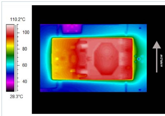
Figure 26 — Thermal plot, 200LFM, 25°C, 48V<sub>IN</sub>, 600W output power
