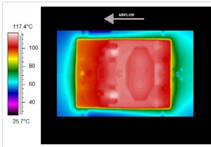
Figure 27 — Thermal plot, 200LFM, 25°C, 48V<sub>IN</sub>, 600W output power
