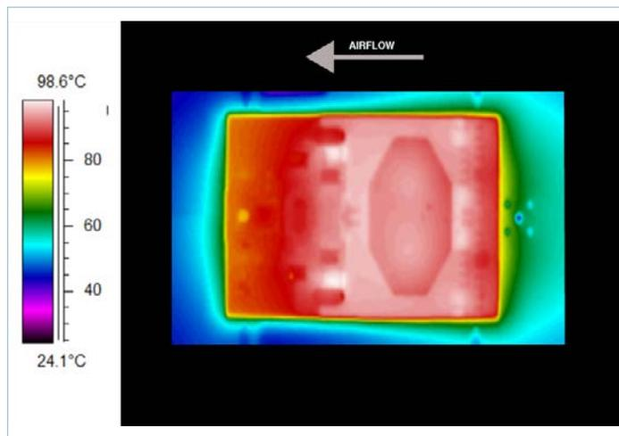
Figure 29 — Thermal plot, 400LFM, 25°C, 48V<sub>IN</sub>, 600W output power
