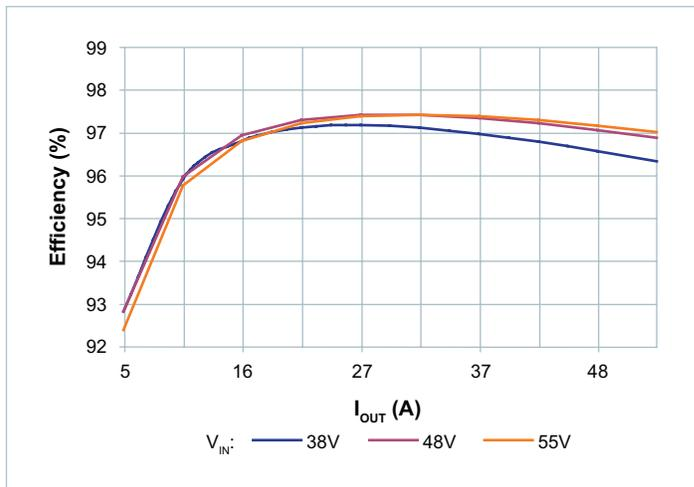
Figure 2 — Efficiency vs. output current, 55°C ambient
