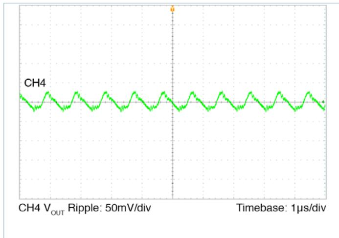
Figure 17 — Output ripple; nominal line, full load
