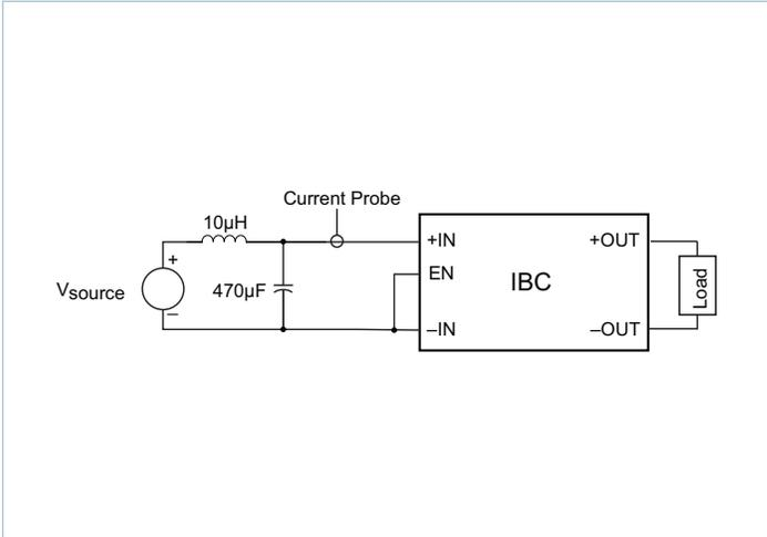
Figure 24 — Test circuit; input reflected ripple current
