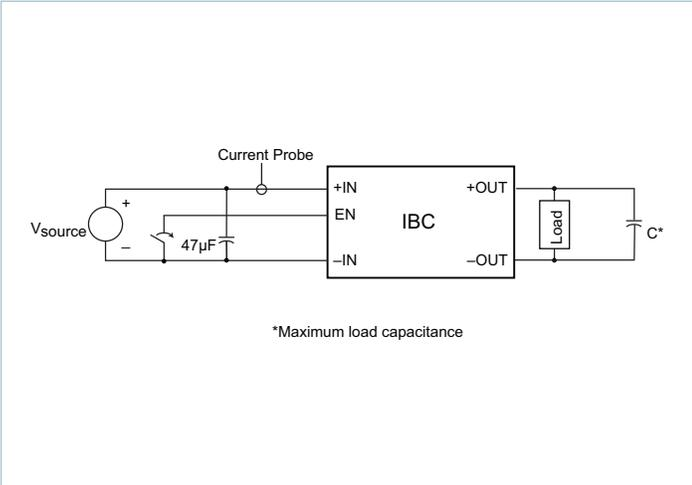
Figure 23 — Test circuit; inrush current overshoot
