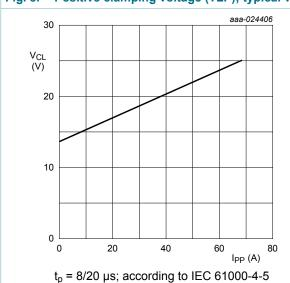
Fig. 10. Positive clamping voltage (8/20 μs pulse); typical values
