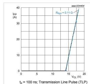
Fig. 8. Positive clamping voltage (TLP); typical values
