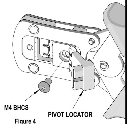
3. Insert the proper terminal fully into the correct profile slot until the terminal is fully seated and stops. Then gently pivot the locator closed.
