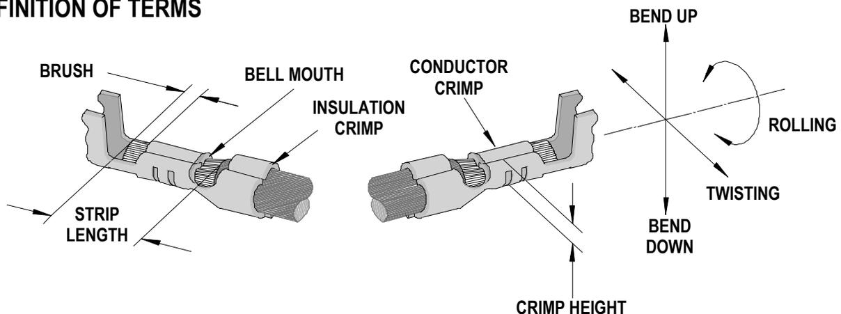
The above terminal drawing is a generic terminal representation. It is not an image of a terminal listed in the scope.
