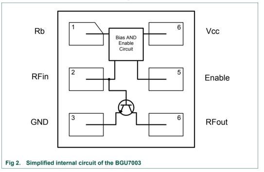
The BGU7003 is not internally matched so for both input and output a matching circuit needs to be designed. The fact that no internal matching is available makes the product suitable for different application areas.
