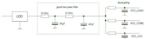
Figure 4.21 Example for a good low pass filtering
