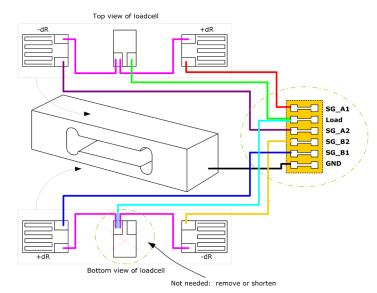
Figure 3.5 Adapted load cell wiring
