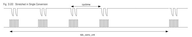
Basically in Single Conversion Stretched mode the parameters remain the same. But tdc\_conv\_cnt defines additionally the time between measurement sequences.
