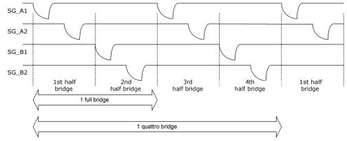
Those numbers of cycles for each mode together define 1 sample (avrate=1). This is also the minimum needed for one complete ratio measurement.
