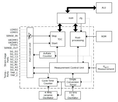
The PICOSTRAIN based converter has the strain gage ports (SG\_Ax to SG\_Dx) to measure:
