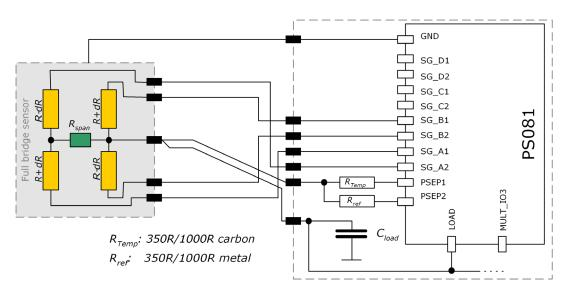
Figure 3.11 6-wire technology with Wheatstone wiring
