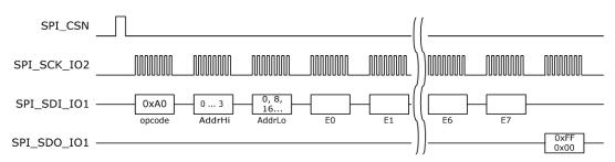
NOTE: EO, E2...E6 are the lower byte, E1, E3....E7 are the corresponding higher bytes in a word.
