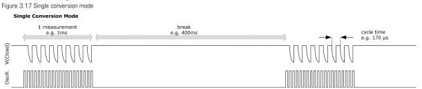
The chip makes a complete measurement sequence and then goes to sleep mode. The oscillator is
