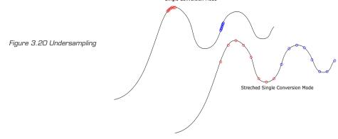
Again, the oscillator is switched on only for each discharge time measurement. But, as the oscillator needs some time to reach the full amplitude, the total active time of the oscillator is longer than for pure Single Conversion Mode. The current consumption in stretched single conversion mode is therefore a little bit increased compared to the single conversion mode.
