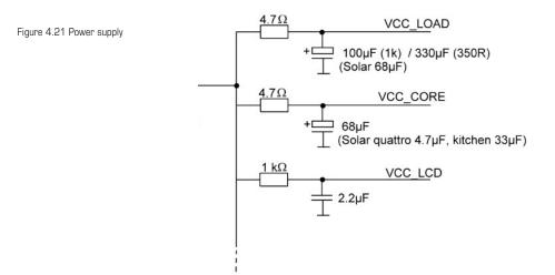
In case of solar applications without any additional battery it is necessary to implement a power-up circuit. It provides a good start-up behaviour when the scale comes from total darkness. A solar panel delivers only a few microampere at poor light conditions and still has to start up the circuit.
