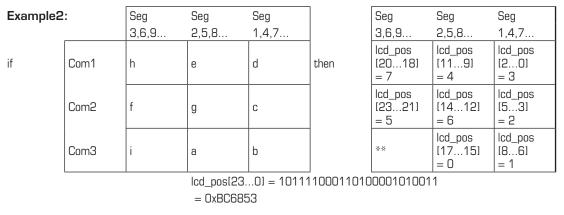
\*\* Special symbols are fixed by LCD design and can not be rearranged. It has to be taken care that those segments are connected to Com3 and Seg3,6,9... Lines
