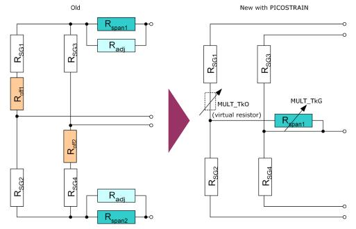
By doing this, the gain and offset behavior of the load cell can be improved by PSO81. This is a very comfortable method to improve the quality of the complete scale without modifying the load cell or the electronic. If this possibility is combined with an intelligent digital load cell concept the production can be simplified at higher quality level and lower cost.
