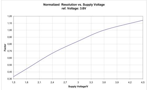
Following diagram shows how the input equivalent noise depends on the supply voltage. The lowest input noise is archived between 2.4 V and 3.6 V. The maximum differential input voltage (e.g. 6.6 mV @ 2mV/V and 3.3 V supply voltage) divided by the input noise gives the effective resolution.
