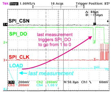
In Fig. 19 you can see that SPI\_DO gives an interrupt after the last discharging cycle of the measurement was done.
