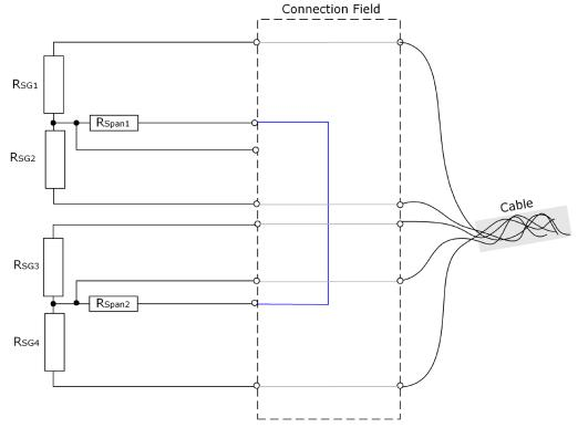
Please note: You are not touching the strain gage sensors or the Rspan resistors directly. Instead you make any re-wiring proposed in the connection field of the load cell. This is true for the changes regarding Rspan as well as the change from Wheatstone-wiring to PICOSTRAIN-wiring (please see also chapter 3.3.2).
