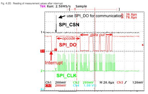
This oscillograph shows again the SPI\_DO interrupt from 1 -> 0 and the response from the external microcontroller with SPI\_CSN. This short pulse on SPI\_CSN switches SPI\_DO to communication mode. Then the opcode is sent to PSO8 (not in the chart, this appears on line SPI\_DI) and after 2 bytes the measurement results (3 bytes) is transmitted via SPI\_DO (marked in the graph by ,data out').
