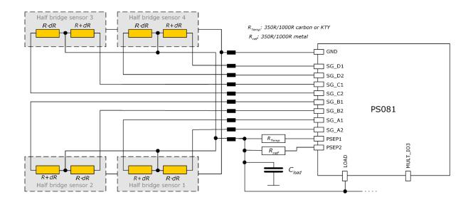
In some cases four sensors are used. Then, each half bridge is connected to one port. This is a typical connection e.g. for quattro body scales. The result of each half bridge can be read but also the overall result.
