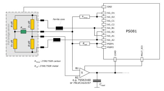
For Wheatstone bridges an additional external analog switch is needed. We recommend TS5A3160 because it has a good behavior even at supply voltages lower than 2.7 V. For supply voltages of 3.0 V or higher 74LVC1G3157 is a good choice, too.
