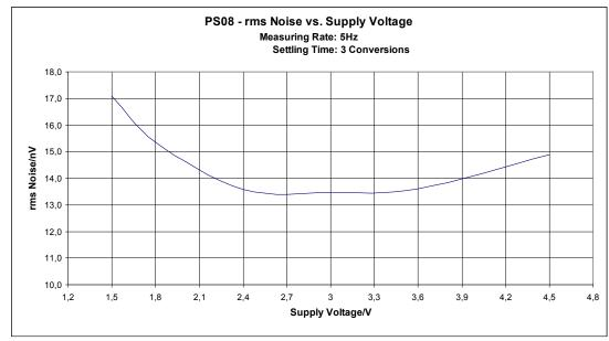
Figure 2.4 RMS-noise vs. supply voltage
