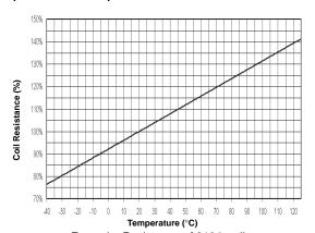
Example: Resistance of  $210\Omega$  coil = 75% of  $210\Omega$  at -40°C, or  $158\Omega$  = 100% of  $210\Omega$  at 20°C, or  $210\Omega$  = 125% of  $210\Omega$  at 85°C, or  $263\Omega$
