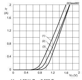
$\begin{array}{l} \text{V}_{\text{o}} = 1.02 \text{ V}; \text{ R}_{\text{s}} = 0.358 \ \Omega \\ \text{(1)} \text{ T}_{\text{j}} = 125 \ ^{\circ}\text{C}; \text{ typical values} \\ \text{(2)} \text{ T}_{\text{j}} = 125 \ ^{\circ}\text{C}; \text{ maximum values} \\ \text{(3)} \text{ T}_{\text{j}} = 25 \ ^{\circ}\text{C}; \text{ maximum values} \end{array}$
