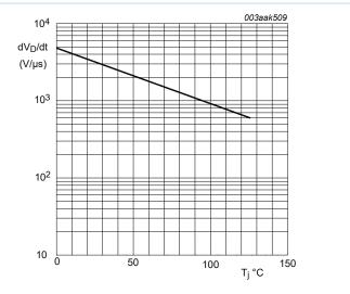
Fig. 12. Critical rate of rise of off-state voltage as a function of junction temperature; minimum values
