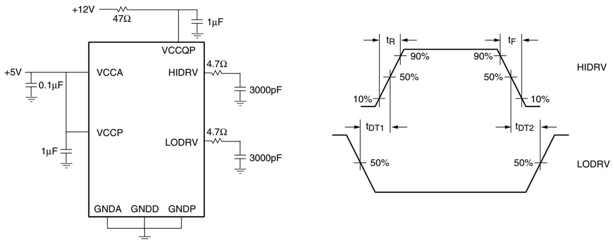
**Figure 3. Output Drive Test Circuit and Timing Diagram**
