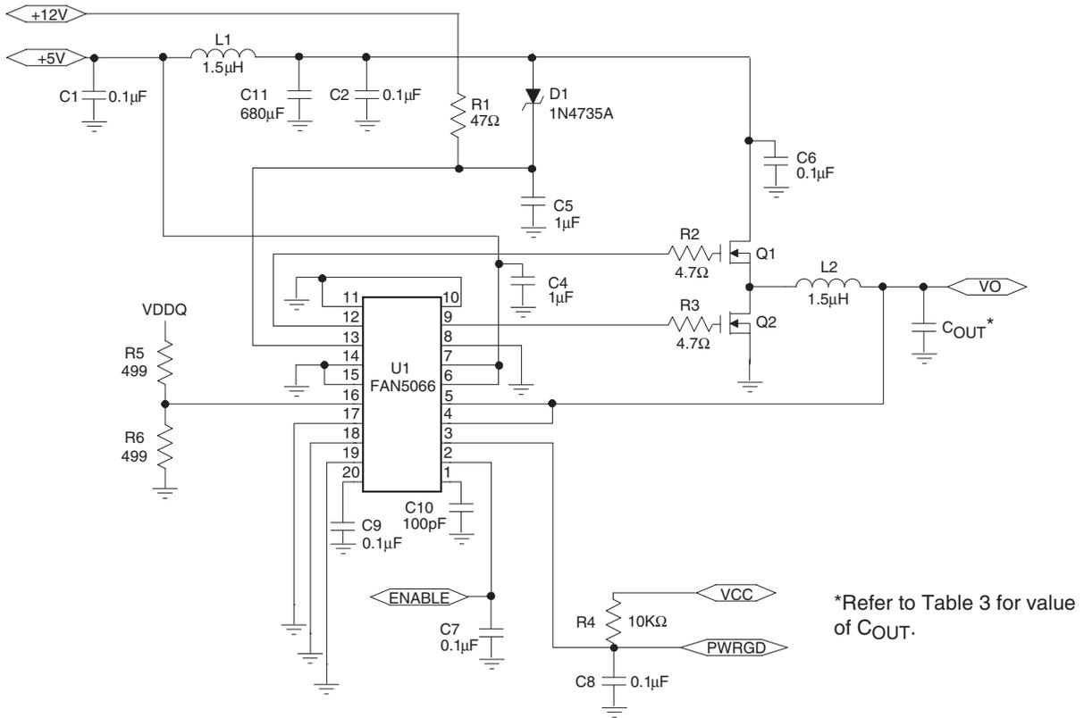
Figure 2. 12A Application Circuit for DDR VTT
