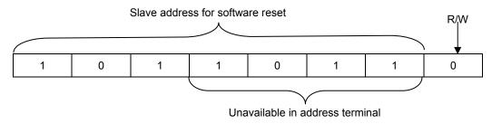
Fig. 7 Slave address for software reset
