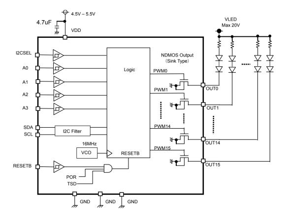
Fig.1 Block Diagram / Application Circuit example
