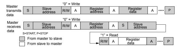
Fig. 4 Basic format of control command (I<sup>2</sup>C)
