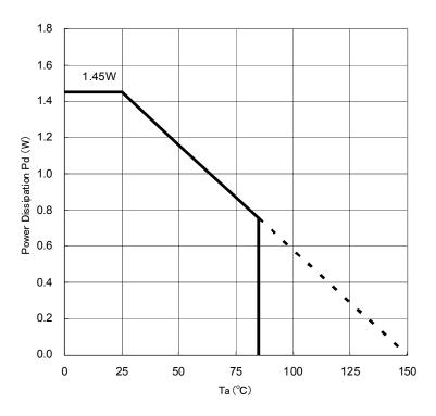
Fig. 9 Power dissipation
