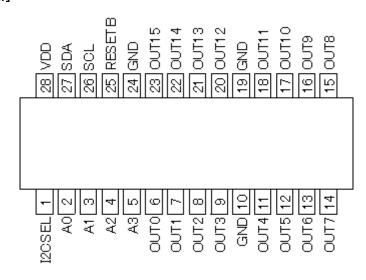
Fig.2 Pin arrangement
