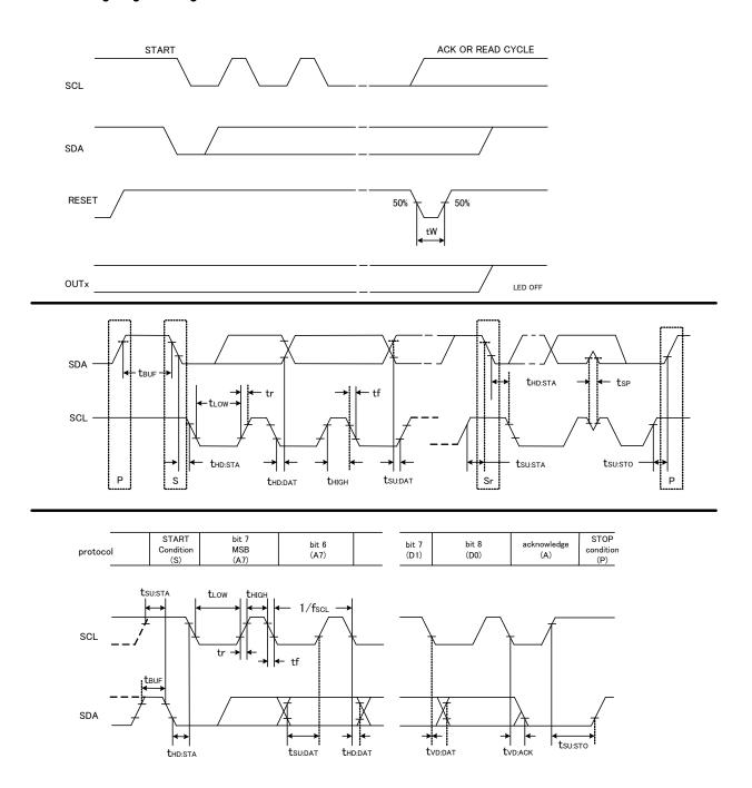
Fig.3 Definition of logic signal timing
