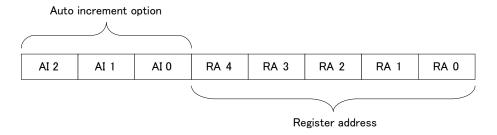
Fig. 8 Register address
