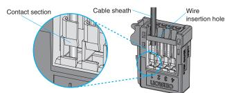
Insert the screwdriver into the release slot, and gently pull back the lever until a click is heard by resetting the lever.
