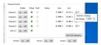
Channels including LDO3.3 can be controlled independently by any GPIO/PSIO or  $I^2C$  command. Channels will start-up or shutdown following transitions of signals applied to GPIO/PSIOs set to control the channels. The control can always be overridden with an  $I^2C$  command.
