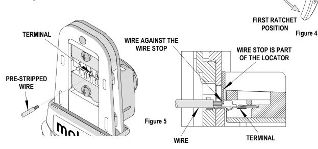
Note: The tamper proof ratchet action will not release the tool until it has been fully closed.
