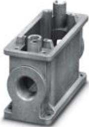
HEAVYCON ADVANCE B16 box mounting base, for M6 screw locking, salt-water-resistant aluminum, with 2 x M32 thread, without surface coating
